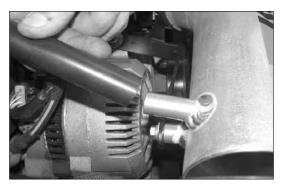
20. Install the crank case vent hose assembly into the 90° fitting at the valve cover and then connect to the vent fitting on the K&N<sup>®</sup> intake tube as shown.
