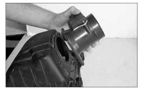
8. Loosen and remove the four bolts that secure the mass air sensor, then remove the mass air sensor as shown.
