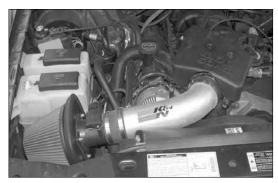
26. Reconnect the vehicle's negative battery cable. Double check to make sure everything is tight and properly positioned before starting the vehicle. 27. The C.A.R.B. exemption sticker, (attached), must be visible under the hood so that an emissions inspector can see it when the vehicle is required to be tested for emissions. California requires testing every two years, other states may vary.
