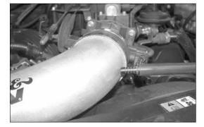
16. On vehicles that come equipped with a second vent line, line up the vent hose on the intake tube and make a mark on the intake tube for drilling.
