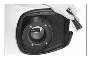
10. Apply the trim seal to the heat shield assembly as shown.
