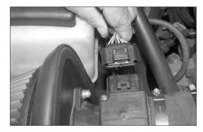
24. Re-connect the mass air sensor electrical connection as shown.
