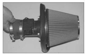
22. Assemble the K&N $^{\ensuremath{\$}}$  air filter onto the heat shield assembly as shown.
