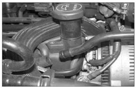
18. Remove the factory plastic crank case vent hose from the 90° elbow on the valve cover as shown.
