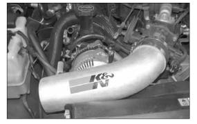
15. Install the K&N<sup>®</sup> intake tube onto the throttle body and line it up with the tube-mounting bracket, then secure with the hose clamp and hardware provided.
