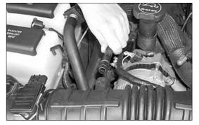
4. Remove the crankcase vent hose from the stock intake tube as shown.
