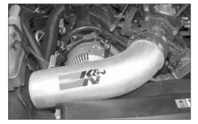
17. Re-install the K&N<sup>®</sup> intake tube onto the throttle body and mounting bracket and then secure with the provided hose clamp and hardware.
