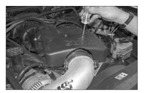
25. Re-install the throttle body cover as shown.
