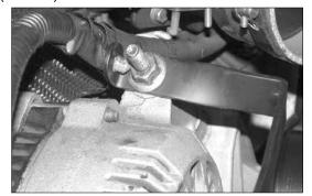
14. Push the wire harness-retaining clip into the hole on the tube-mounting bracket as shown. **NOTE: Be sure the wire harness is clear of the throttle linkage.**
