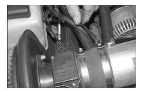
11. Assemble the silicone hose (08051) and the hose clamps onto the heat shield assembly as shown.
