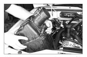
7. Using a screwdriver, pry up the bottom of the air cleaner to release the air cleaner from the stock grommets, then remove the air cleaner assembly as shown.
